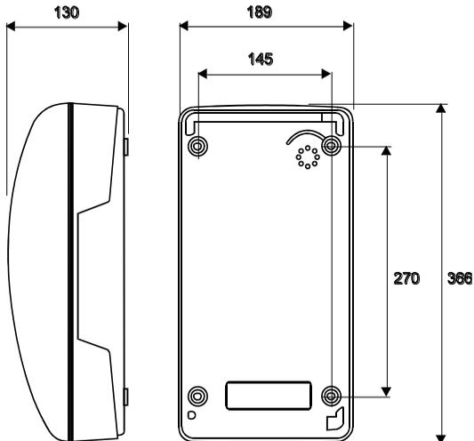
1. Using a suitable tool, punch out 4 holes in the rear enclosure, taking care not to damage or dislodge the plastic bushes. Only four of the eight holes are required - the outer ones are recommended. The
