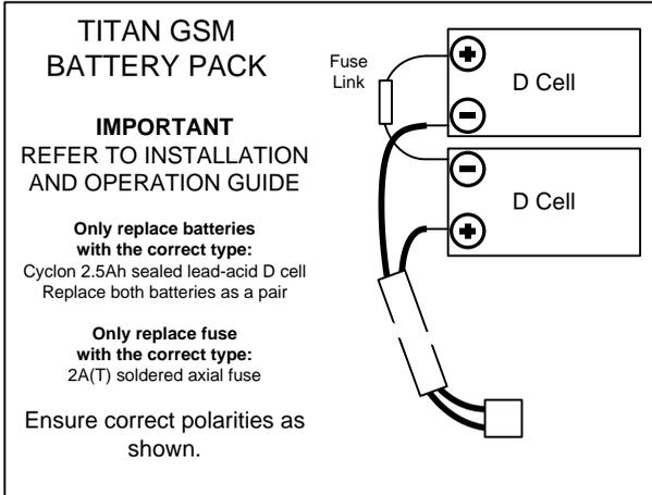
Always ensure the batteries are connected before connecting the power supply, or the batteries may not charge.
