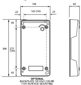
When wall or pole mounted, VR and Help Point units must be fitted inside a dedicated rear enclosure.
