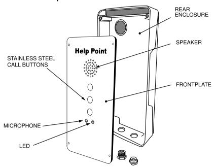
This manual describes Help Point and VR (Vandal Resistant) ranges of hands-free telephone products. These units offer high degrees of resistance to weather and abuse, having only a microphone, speaker and one or more metal buttons mounted on a flat, metal faceplate, in place of a traditional handset and keypad. Main features include:
