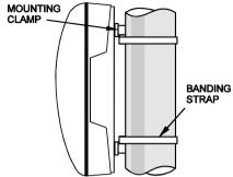
This accessory is for mounting GAI-Tronics telephones on to the side of round poles of 100mm to 200mm diameter, or on to square or rectangular section uprights of 100mm to 150mm across the mounting surface.
