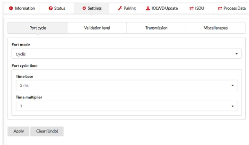
Figure 26: Settings tab, Port cycle sub tab (example)
