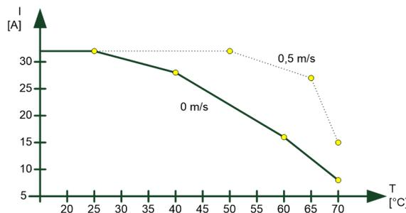
Figure 3: Derating netFIELD IO-Link Wireless Master device
