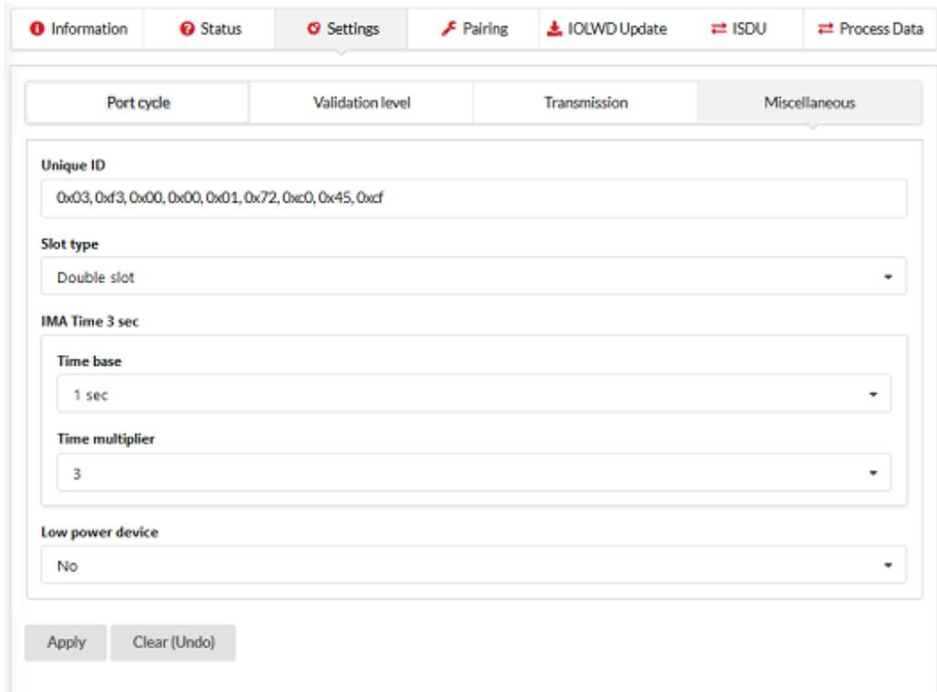
Figure 29: Settings tab, Miscellaneous sub tab (example)
