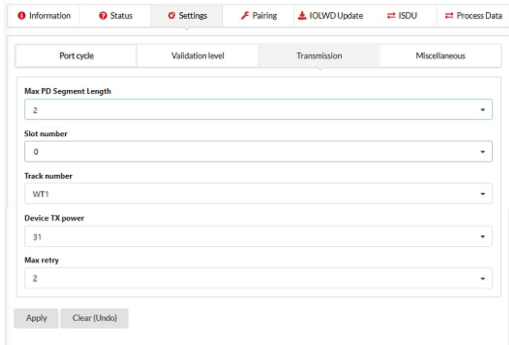
Figure 42: Settings tab > Transmission sub tab (example)
