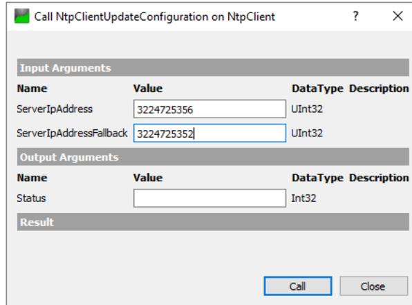
Figure 51: Dialog for configuring the NTP client
