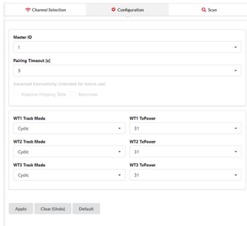
Figure 21: IO-Link Wireless Master > Configuration tab
