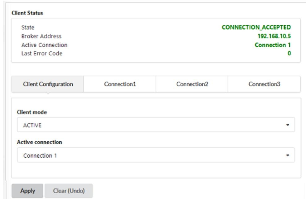
Figure 14: MQTT tab, Client Status, Client Configuration sub tab (example)
