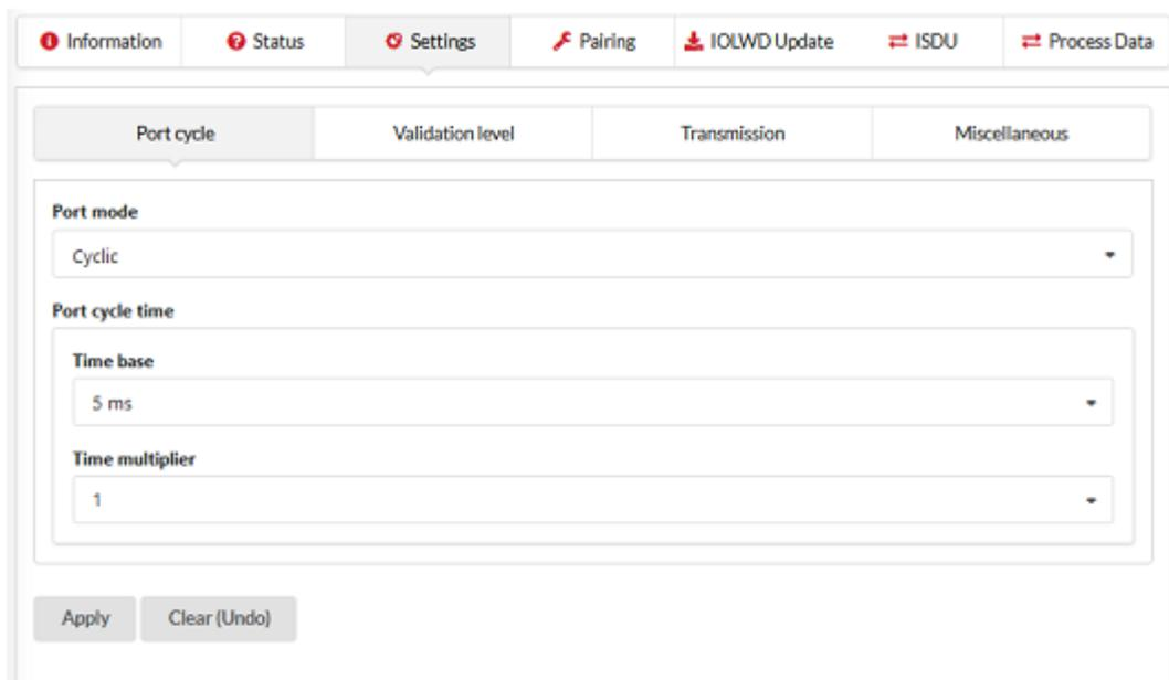
Figure 40: Settings tab > Port cycle sub tab (example)
