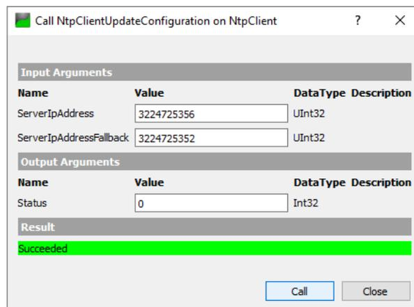
Figure 52: Dialog for configuring the NTP client (successful)
